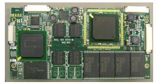
The intent is for it to be used as a computing component, with some add-on hardware for whatever you specifically need - power management, GPS, camera, motordrivers for robotics, etc. A number of boards have been made by Cambridge University Engineering Dept for their robotics and computing teaching courses.
